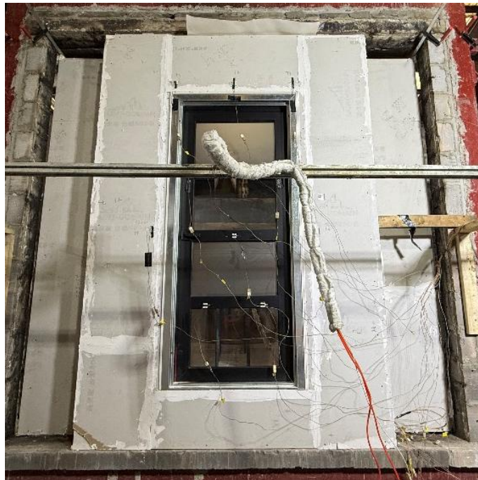
Fig. 4 Non-fire exposed side after 60 minutes
