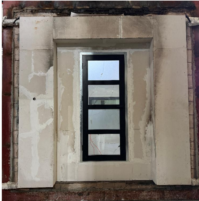
Fig. 1 Fire exposed side Prior to the radiant heat test
