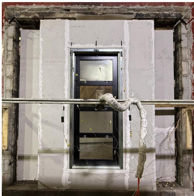
Fig. 2 Non-fire exposed side Prior to the radiant heat test
