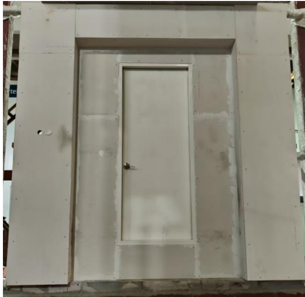
Fig. 1 Exposed Side before the Radiant heat test
