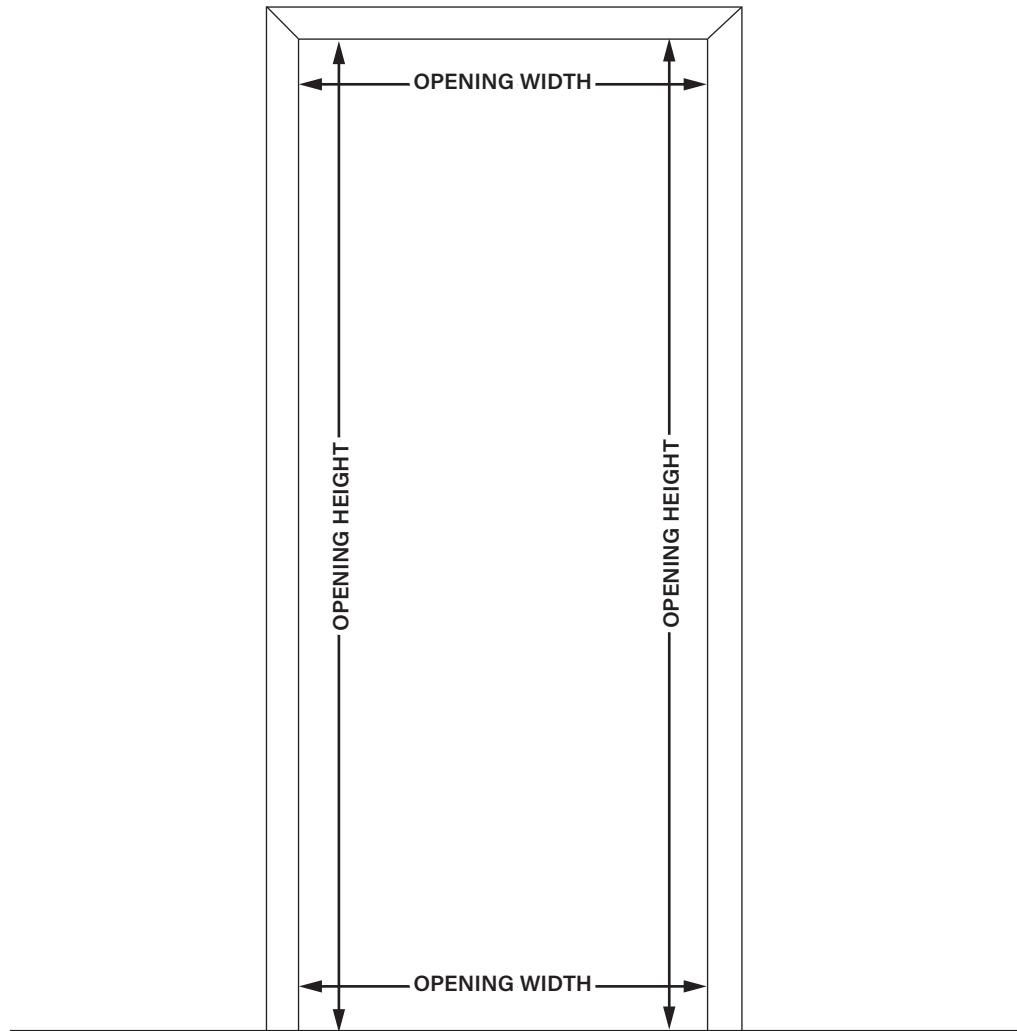
\* Measure door opening before installing.
