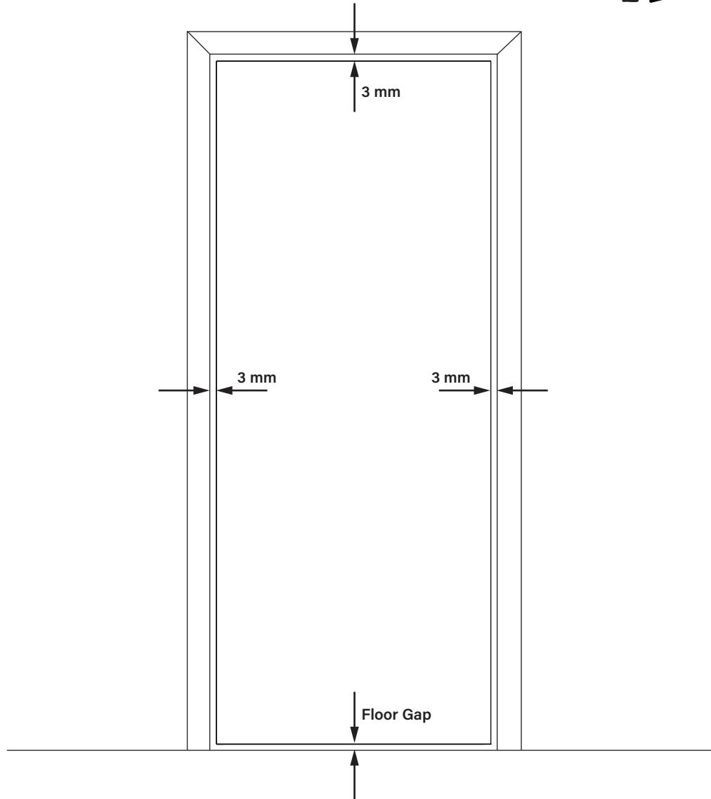
**i** DOOR WIDTH = opening width - 6 mm (allowing 3mm clearance on each side)
