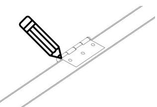
**Step 2:** Chisel or router hinge area making sure not to cut deeper than hinge thickness.
